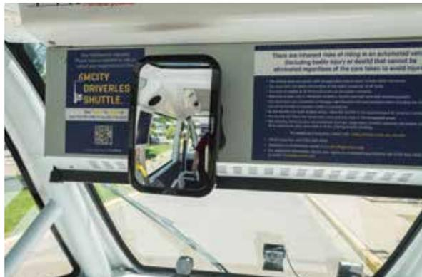
**A mirror located inside each shuttle helps the on-board safety conductor see what's happening behind them.**
