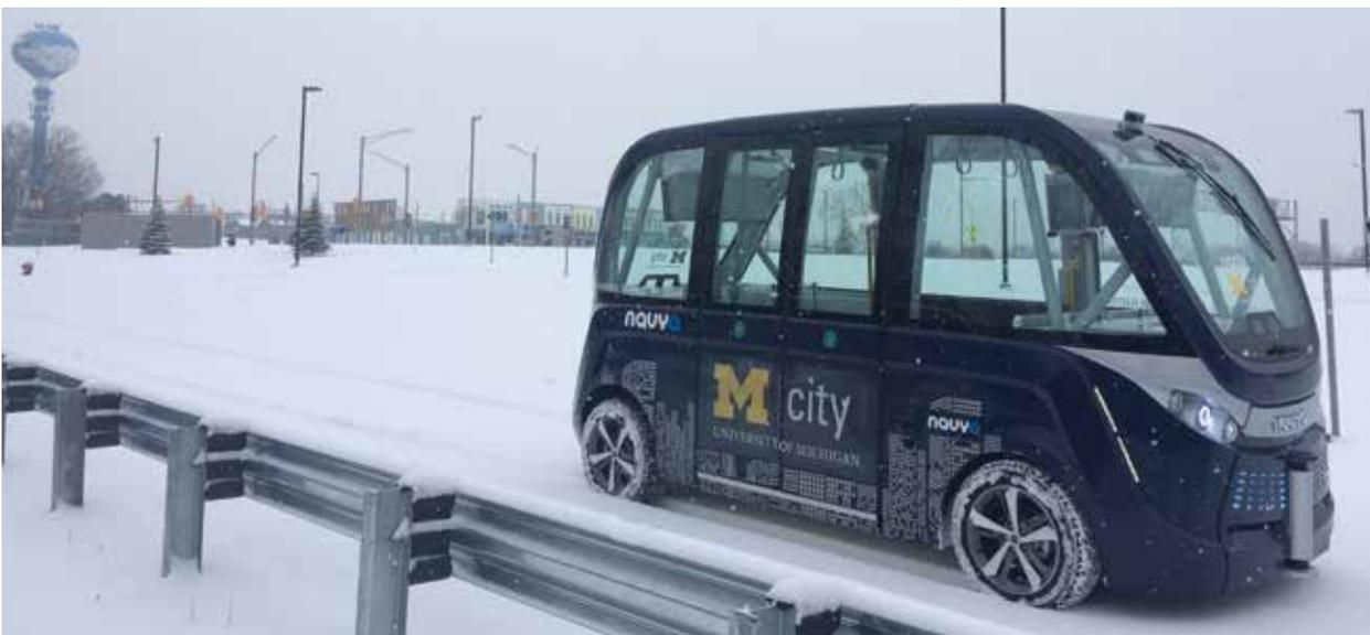
**Mcity evaluated the performance of a NAVYA driverless shuttle for over a year in a variety of weather and lighting conditions inside the Mcity Test Facility.**
