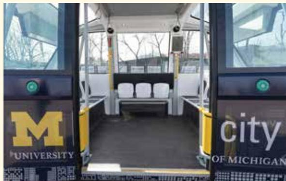
**The Mcity Driverless Shuttle project uses two NAVYA Automon electric shuttles.**
