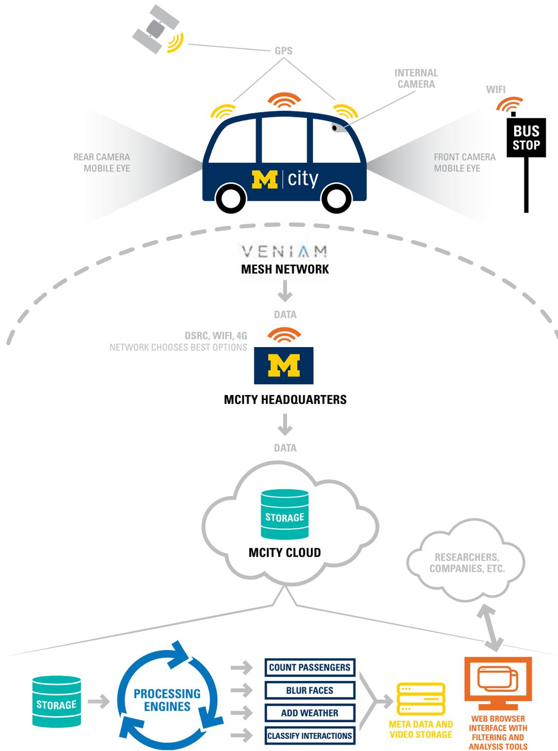
The Veniam mesh network used by the shuttles collects, synchronizes and transmits data to Mcity's cloud systems for later processing.
